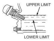
Figure 4. Engine Oil Dipstick
